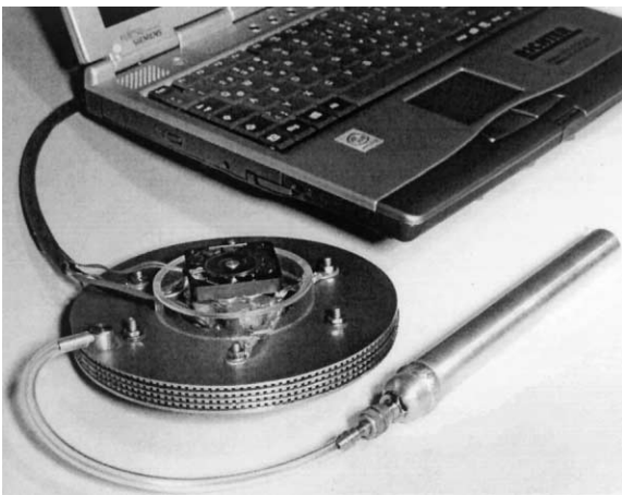
Fig. 5. Fuel cell stack with four cells and 55 W maximum power connected with a dc-converter to deliver 3.5–15 V.
